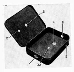
Refer to the text for dimensions of the holes drilled in the hinged metal box shown above. After drilling, deburr the holes and, after preliminary wiring, mount and finish wiring the components as shown at the right.
