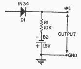
Fig. 5. Equivalent circuit for off signal.
