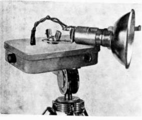
The completed slave photoflash can be mounted on a tripod as shown here. Enough twisted lead is left so the flash can be swiveled in any direction by loosening the wingnut.
