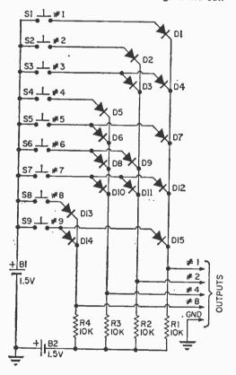
Fig. 3. Diagram of a matrix circuit capable of positive (on) and negative (off) signals.
