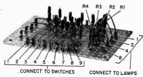
Bare copper leads suspended between flea clips serve as busses to form the matrix.
