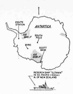
Map of Antarctica shows locations of VLF receiver stations for the propagation tests.
