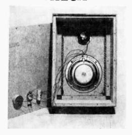
The completed speaker kit (left) is ready for its fiberglass stuffing. Now is the time to check your wiring. Below, a coat or two of clear lacquer will protect the oil stain finish.
