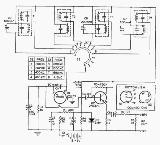
Frequency determining tank circuits are selected by switch \$2 and passed to collector of Q1.
