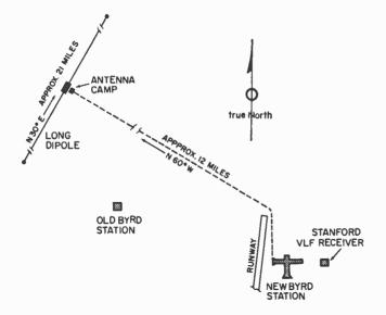
Sketch of the Byrd Station area shows the location and orientation of the dipole along the magnetic meridian 30° east of true north.
