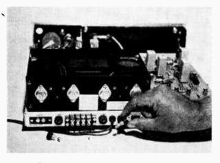
Chassis layout is neat and clean with all parts exposed from the top. In kit form the EICO 3566 offers no assembly problems.
