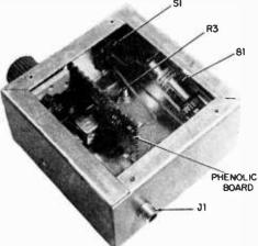
Board mounts vertically in case, held in by the tuning capacitor. BFO signal is at J1.
