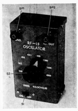
Large indicator knob with pointer and front panel decal markings allow for quick and easy selection of the desired fixed frequency.
