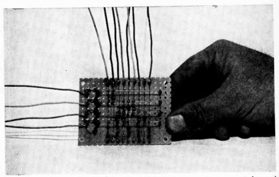
A simple rectangular array of semiconductor diodes plus some switches and lamps can be assembled by you to convert decimal numbers to binary digits
