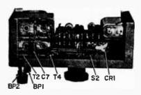
Side view of the unit shows grouping of IF cans held by the fabricated metal bracket. Carefully drill four holes in back half of the cabinet for tuning the cans with the back on.
