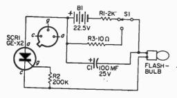
Cut two lengths of insulated hookup wire about 8 inches long. Twist them together to make a two-wire lead. Feed the twisted lead through hole 2 in the case lid. Fasten one of the wires to the cathode lead of SCR1 and solder. Solder the other wire to the pole of S1 where the negative lead of C1 is attached.
