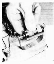
Bulb is quickly tested using the test prongs attached to the first two Fahnestock clips. The 1.5 volts is enough to check for an open filament. Flashlight cells are checked in a flash in the fabricated bulb holder and strip. Brightly lighted or dimly lit bulb indicates strength.
