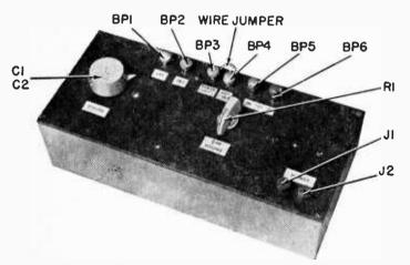
Front-panel view shows tuning and volume knobs. Binding posts along top edge are for connecting battery, antenna and jumper. Use a red post for BP6, black one for BP5. Other posts are white. Output is obtained at jacks J1 and J2.
