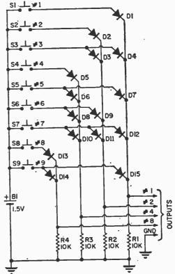
can be eliminated (shorted out) and their inputs connected directly to the outputs because neither the diode's isolation or resistance is needed in this circuit.
