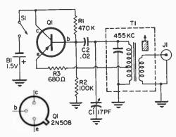
Be sure to follow Q1 connections, as shown in schematic above. Q1 mounts in transistor socket seen in left photo. Wire complete board before inserting in metal case.
