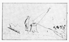
Diagrams from Loomis' notes record for posterity the equipment setup used in 1866. Above, receiving station consists of detector on log, antenna suspended by kite and ground wire in lake; below, identical setup, however, antenna is connected to detector to trigger impulse.
