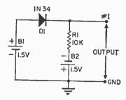
Fig. 4. Equivalent circuit for on signal.
