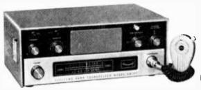
• 5 crystal-controlled transmit & receive channels • Receives all 23 channels • Built-in 4-tone selective call • Tuning meter • Adjustable squetch • Built-in 3-way power supply—6 or 12 v. DC, 117 v. AC • PTT mike, power cables & crystals for 1 channel. 23 lbs.
