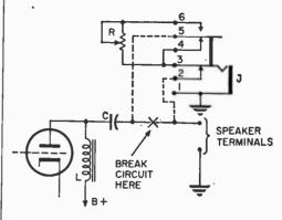
chassis or cabinet, break the circuit at X in the diagram and add R, a 10,000 ohm potentiometer, all connected as shown. When the phone plug is inserted in the jack, its 4-5 and 2-3 contacts open, disconnecting the speaker. Its 5-6 contacts connect the audio output to the ungrounded headphone lead (tip of phone plug) through R which is connected as a series rheostat and serves as a headphone volume control.
